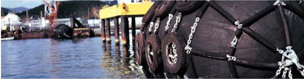
This is ideal in the situations where a fixed fender is not applicable such as to ship-to-ship operations off shore and some ship-to-wharf operations. It is also suitable for the use at a quay where the tidal range is large. Like the hollow cylindrical fender, its initial reaction load is low at the early stage of compression and its cushion effect is virtually independent from an approaching angle of a ship. Size range: 0.3~3.3m o/d
